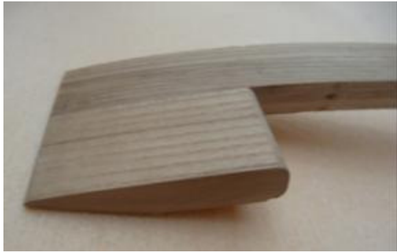
This is the leg and foot joined together after being planed and sanded to give a smooth finish.
