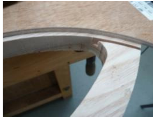
Then they made a wooden template the same shape of the curve so that the follower router could follow the template to cut out a halving joint in the wood so that the metal could slot inside.
