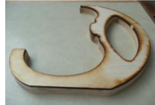
This is the main body cut out with the template still attached to it.
