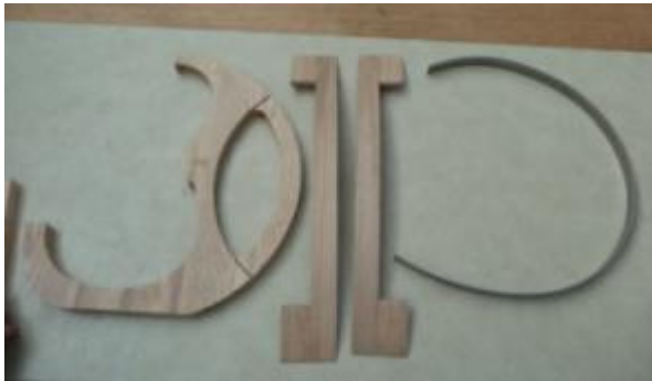
I over estimated the amount of work to complete in my project, so that I could finish my teacher and the technician made and fitted the metal curve of my work for me. They first bent a piece of strip aluminium metal around a metal former.
