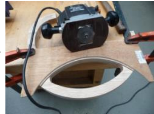
They used the follower router to follow the template to cut the joint exactly.
